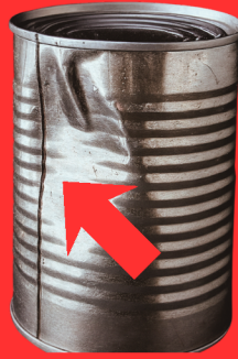
Dent over side seam
