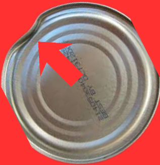
Dent over end seam*
